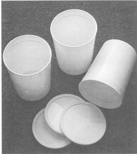
FIG. 1—The containers are 19.05 mm (7/2 in.) tall, 146.05 mm (5¾ in.) wide at the mouth, and 120.65 (4¾ in.) wide at the base. They have a snap top lid. The top is low density polyethylene and approximately 0.81 mm (32 mil) thick. The body of the container is high density polyethylene and approximately 1.27 mm (50 mil) thick. They are from Reb Plastics, Inc., Avon Lake, OH.
